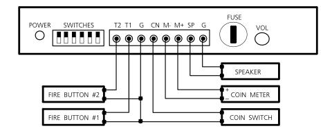
EM2021D is a highly reliable controller box designed for use in coin operated kiddie rides with the following features:
