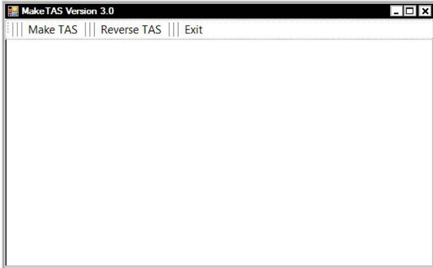
Click [Make TAS], navigate to and open the schedule file. The TAS file will then be generated and placed in the same folder if there are no errors. The TAS file has the same filename as the schedule file but with TAS\_ added to the beginning. For example, the TAS file for abc.txt is TAS\_abc.txt. Note that although the TAS file has a txt file type it's not a text file anymore.
